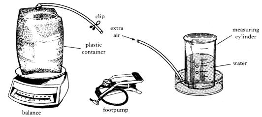
Using the footpump, extra air is pumped into the container. This extra air is released into the measuring cylinder as shown above and its volume measured. The following measurements are recorded.
