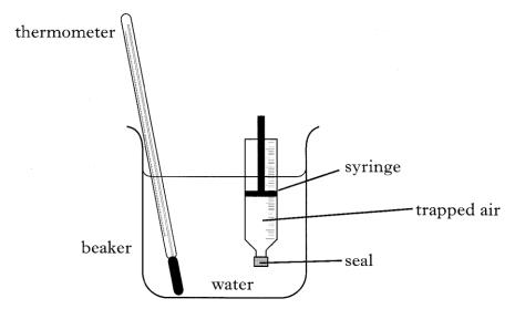
The volume of the trapped air is read from the scale on the syringe.
